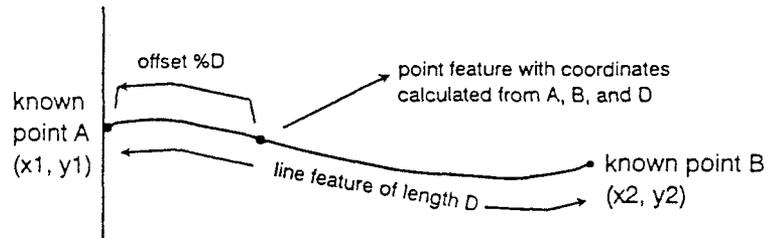
**Fig. 2.2 Linear Referencing Methods**
